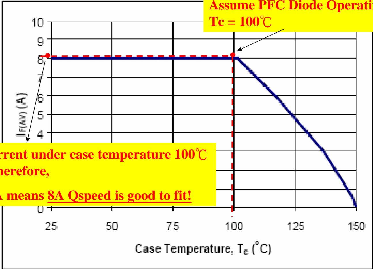
**The DC Current under case temperature  $100^\circ\text{C}$  is 8A, and therefore,
