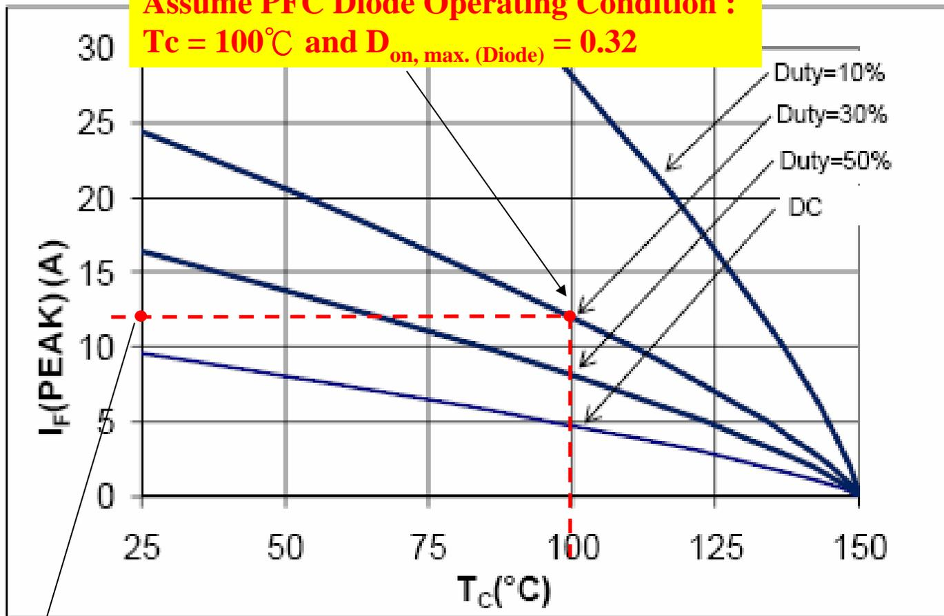
**LQA03TC600  $I_F(\text{PEAK})$  vs  $T_c$ ,  $f=70\text{kHz}$ .**
